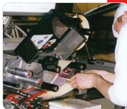
With ALX 924 labels can be replaced without stopping the production line
